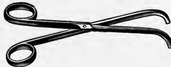
FIG. 4. SHORT CRUCIBLE TONGS.
