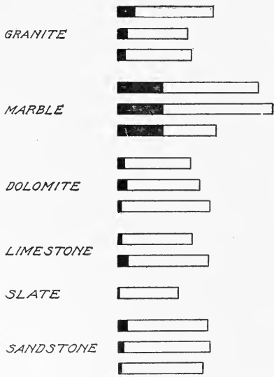
Fig. 80. Diagram Showing Relative Permanent Expansion of Different Building Stones After Heating to a Temperature of About 400° to 440° F.
