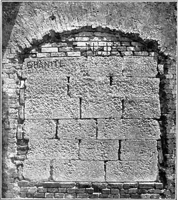
Fig. 115. Appearance After Test of Panel Containing Granite-Concrete Beams
