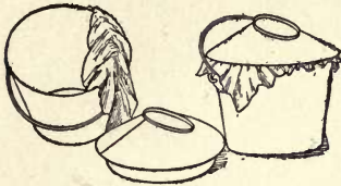
COMBINED STRAINER AND SMALL OPENING MILK PAIL. DR. NORTH'S STYLE.
