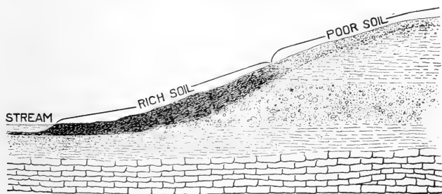
Diagram showing the movement of the soil from higher to lower levels
