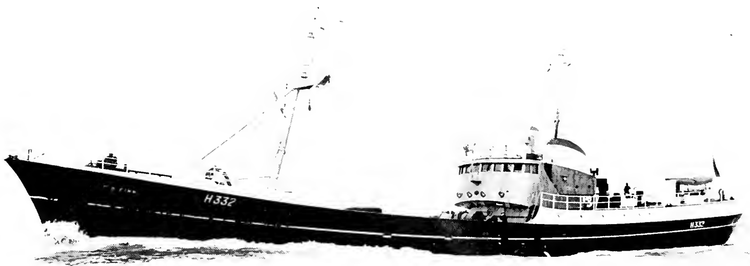
M/V D. B. Finn , 202-foot, deep-water, conventional trawler, fishes Iceland, Barents Sea, Bear Island, Greenland, and all distant Arctic grounds.
