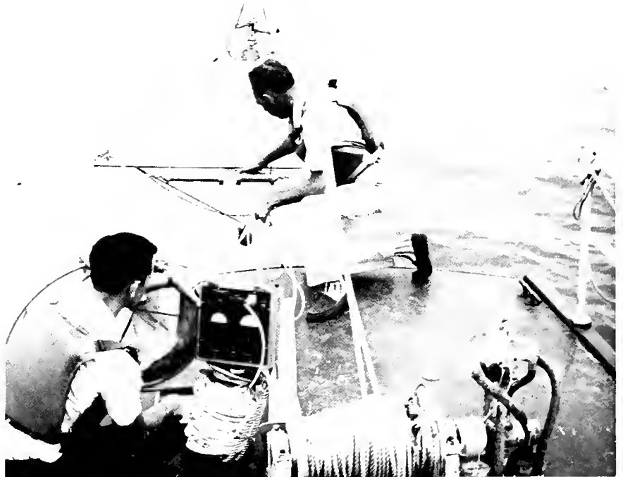
Biologist uses a light transparency meter to measure turbidity in the waters of Galveston Bay, Tex.
