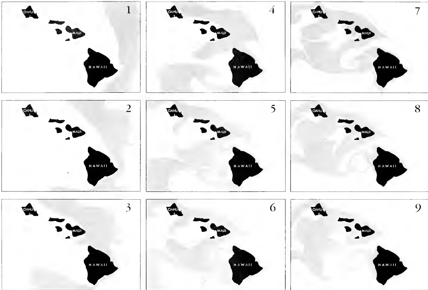
FIGURE 20. The 363,000 square miles of the Howoiiion areo have been shrunk to the size of a large pool table in a three-dimensional scale model at the Laboratory in Honolulu. By injecting dye into the water, scientists can study the development of eddies in the lee of the islands. Here is an artist's rendering of one such experiment,
