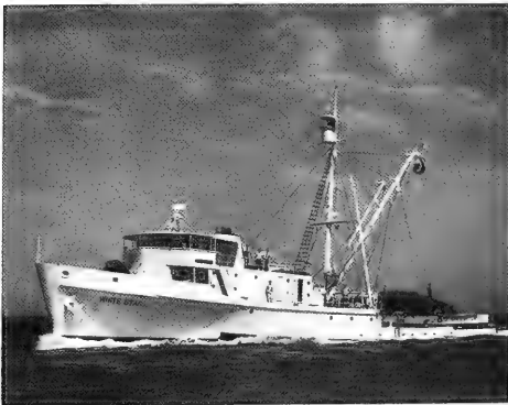
THE SAME VESSEL AFTER CONVERSION TO A PURSE SEINER.
