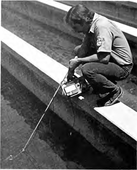
FIGURE 39. An essential instrument in any fish rearing operation is an oxygen meter. Catastrophic fish losses can be avoided if oxygen concentrations are checked periodically and the optimum carrying capacity of the hatchery can be determined. Several brands of meters are available commercially. (FWS photo.)
