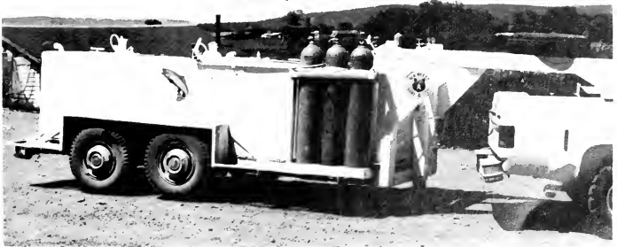
FIGURE 108. Fish distribution tank mounted on a gooseneck trailer. This unit can be pulled by a pickup truck.
