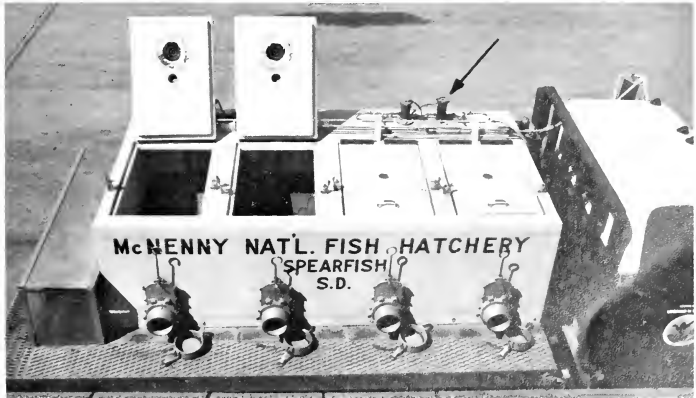
FIGURE 109. Fiberglass distribution tank with four compartments, each with an electric aerator (arrow). Additional oxygen is provided through carbon rods or micropore tubing on the bottom of the tank. (McNenny National Fish Hatchery, FWS.)
