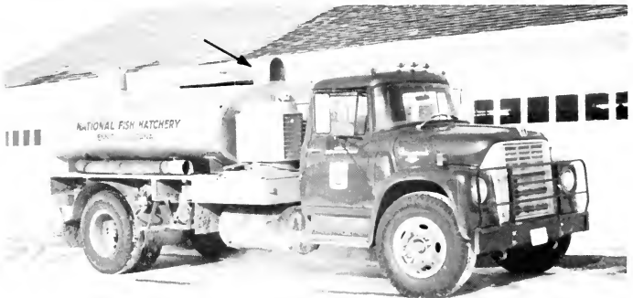
FIGURE 111. Aluminum elliptical tank with refrigeration unit mounted at the front. Aeration is by gas-driven pumps and pure oxygen. Note air scoops (arrow) for CO 2 removal on front and rear of tanks. (Ennis National Fish Hatchery, FWS.)
