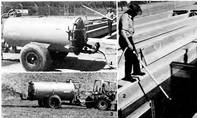
FIGURE 15. (1) A vacuum liquid manure spreader with a modified hose connection can be used to remove settleable waste solids from fish rearing units. (2) Water flow is controlled with a \frac{1}{4} -turn ball valve (arrow). The valve is shut off whenever the cleaning wand is not actually drawing up waste. Note the settling area provided at the lower end of the raceway. (3) The collected waste solids are then spread on agriculture lands or lawn areas away from residences. (FWS photos.)
