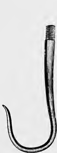
FIG. 1. INCORRECT FORM OF GAFF.
