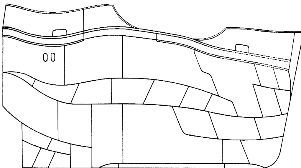
Fig 35. Shell profile of a British steel chine boat
