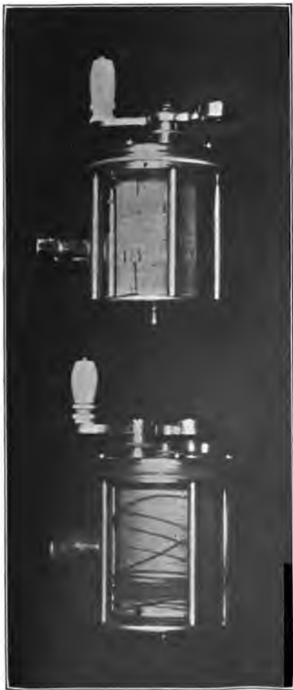
Fig. 8—Reels of Same Size Fitted With Cork Drums, 1\frac{1}{2} inch in Diameter, Actual Weight of Cork Being About 30 Grains. Right-Hand Reel Shows Cork Drum, and Left-Hand 100 Yards of Tournament Line, on Drum and 7 foot Heavy Silk Leader
