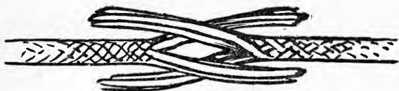
Fig. 28.—Frayed Ends of Line Ready for Splicing.
