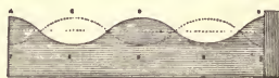
FIG. 20. Water-wave in dotted outline neutralises wave in continuous outline, producing level surface.
