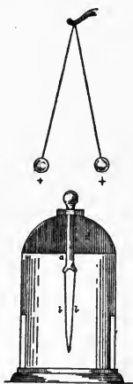
FIG. 24. Electrical repulsion and attraction.
