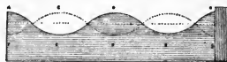
FIG. 20. Water-wave in dotted outline neutralises wave in continuous outline, producing level surface.
