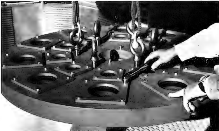
Figure 12. Flange for simultaneous proof testing of 20 EDU windows.
