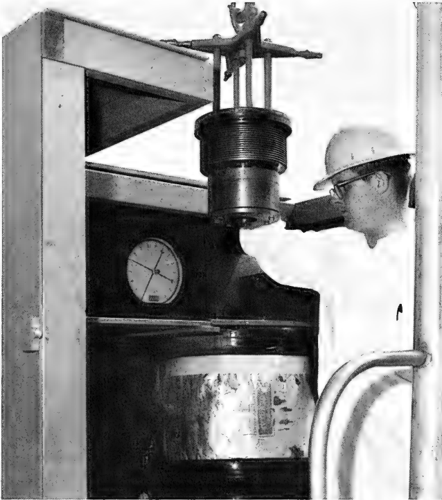
Figure 4d. Lowering the end-closure assembly into the pressure vessel.
