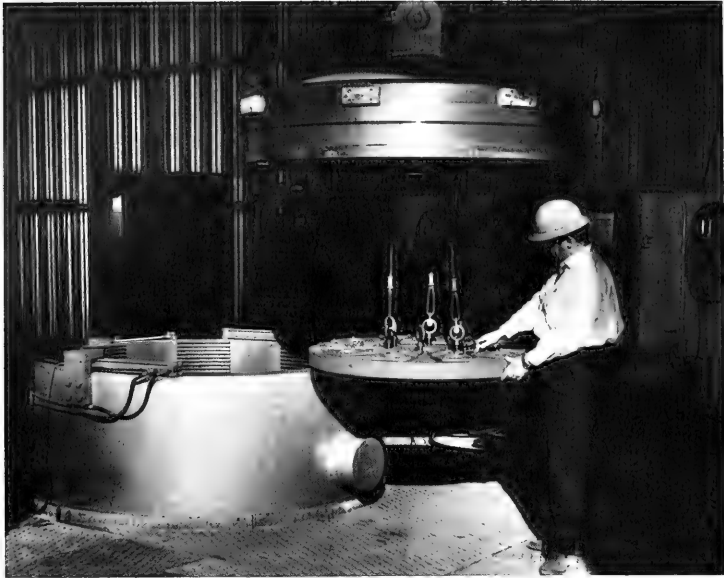
Figure 11. Arrangement for proof testing of EDU windows in NCEL's 72-inch diameter pressure vessel.
