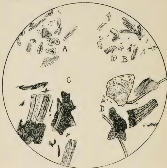
FIG. 10.—Micrograph showing appearance of (A) Ground Coconut Shell, (B) Ground Olive Stones, (C) Wood Dust and (D) Cocoa Shell Powder.
