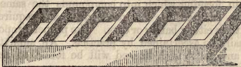
Fig. 18. —Mould for Linseed compound.
