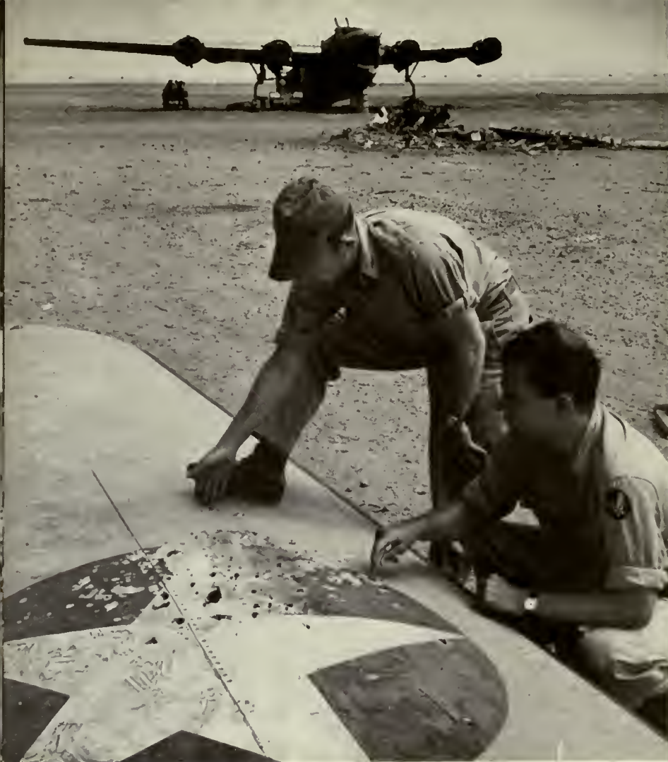
Patches, rivets, and paint will repair Nazi damage to American star. If other parts are needed, cannibalized "Battle Ax" in background can provide them.
