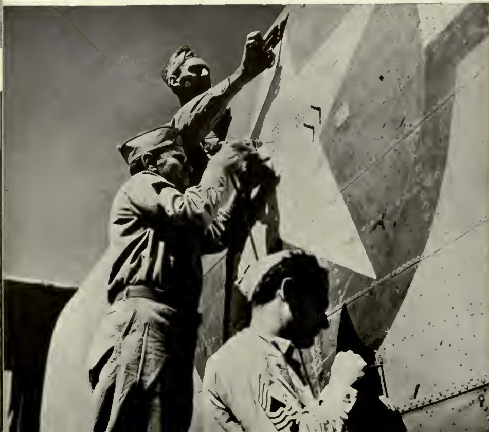
Patches, rivets, and paint will repair Nazi damage to American star. If other parts are needed, cannibalized "Battle Ax" in background can provide them.
