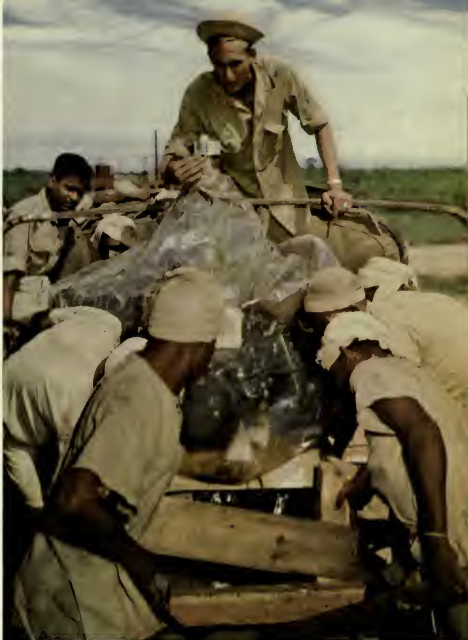
Airplane engines arrive in Assam "pickled" in grease and wrapped in Cellophane. (below) Lieuts. Willis, Lichtenfels, and McCall watch loading of bombs for China.
