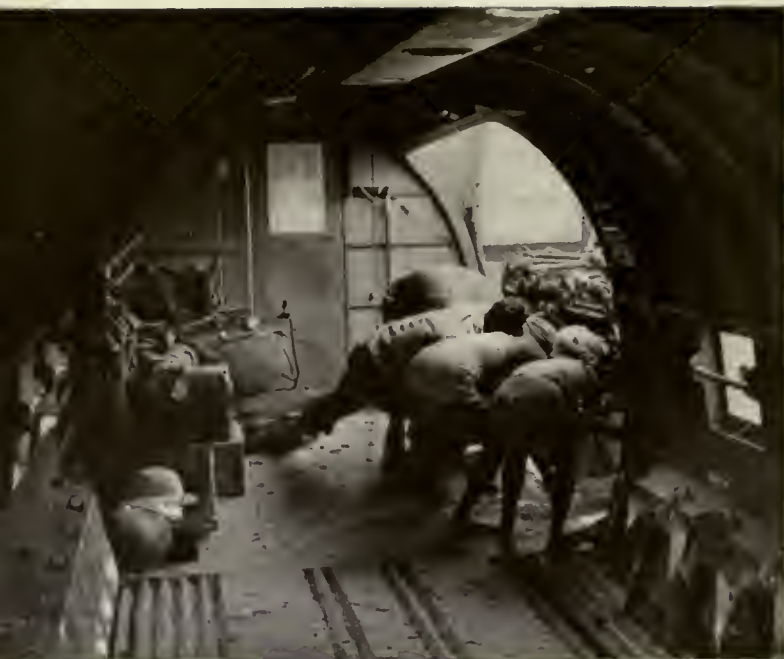
COLLAPSIBLE BUCKET SEATS ARE DROPPED TO MAKE ROOM FOR CARGO
