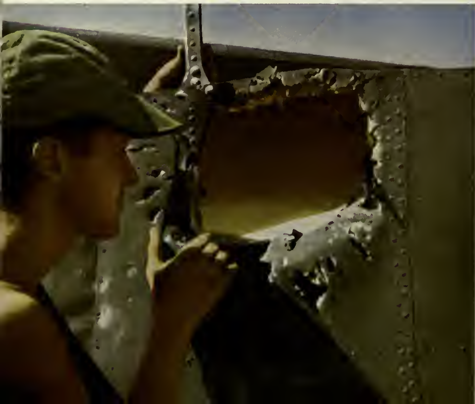
Sgt. Lewis M. Shields and T/Sgt. Chas. J. Cammock check damage to "Daisy Mae's" tail turret. Sturdy Liberators return in spite of huge flak holes like this.
