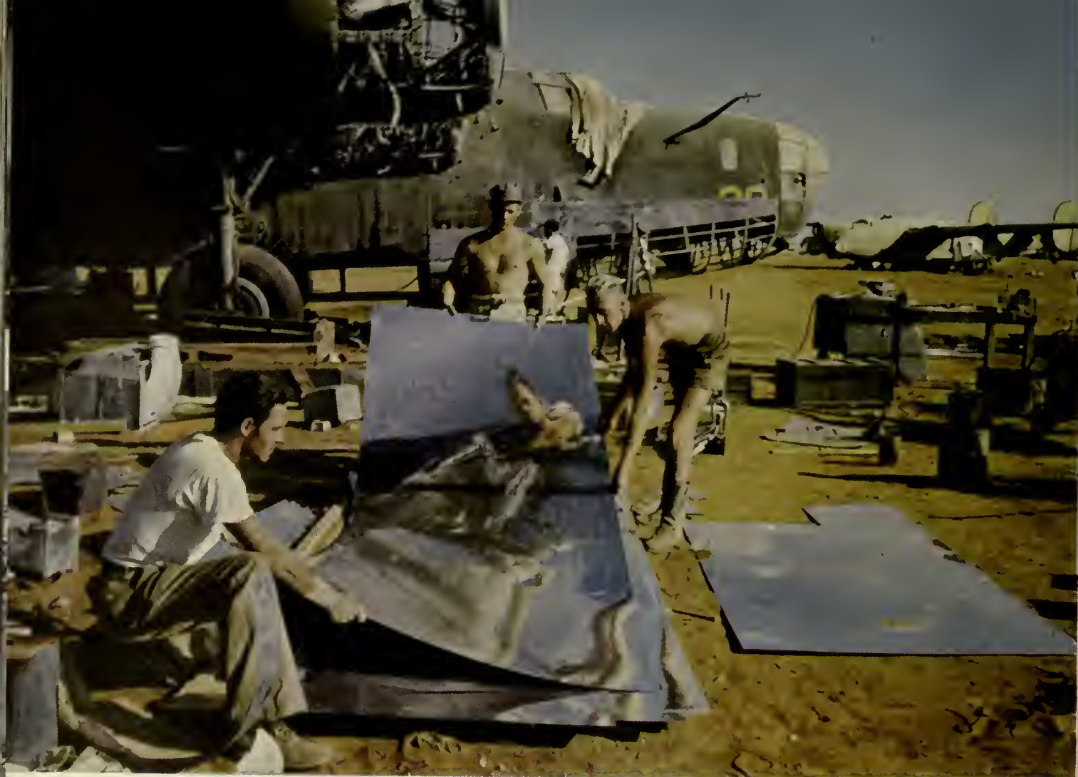
↑ Open-air workshop. Sheet Duralumin, portable workbench, handmade jigs plus ingenuity quickly restore wrecked planes.
