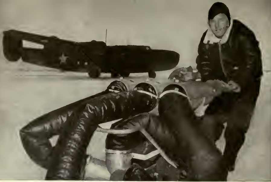
Mechanic thaws chilled fingers in warm air blown from portable gasoline heater, indispensable for the subzero maintenance work. (below) Labrador farewells.
