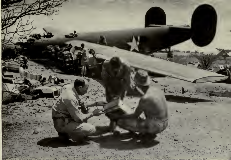
Cargo ships, too overburdened for take-off, occasionally belly-land at end of runway. Crew under civilian John W. Byrnes (left) quickly makes repairs.
