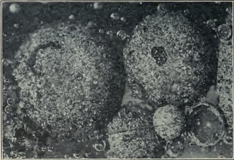
FROTH WITH 0.1% OIL, MAGNIFIED 400 TIMES
