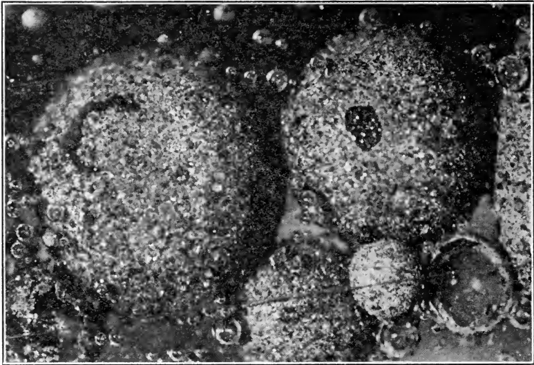
FROTH WITH 0.1% OIL, MAGNIFIED 400 TIMES
