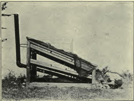
A HOME-MADE DRYING OUTFIT THAT IS PRACTICAL AND INEXPENSIVE; ON WARM, BRIGHT DAYS A FIRE IS NOT NECESSARY
