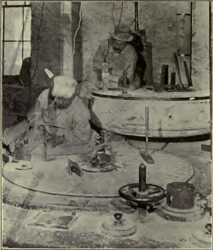
Fig. 9.—Roughening Burr-Stones. (Courtesy of the Washburn-Crosby Co.)
