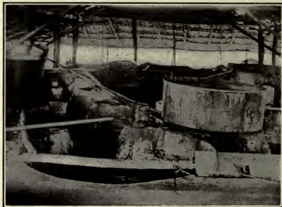
Fig. 33.—Open Pan Evaporators, Philippines. (Courtesy of the School of Mines Quarterly, Columbia University.)
