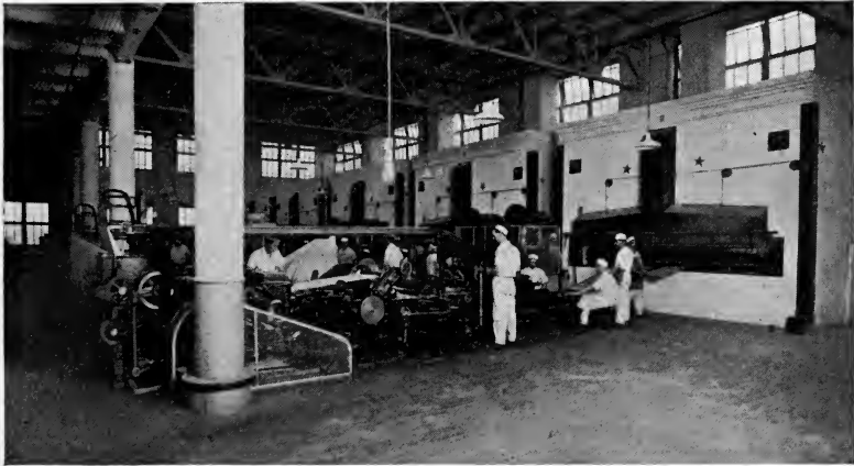
Fig. 24.—Baking Floor for Sweet Goods showing Sweet Cracker Machine and Pans being placed in the Oven. (Courtesy of National Biscuit Co.)
