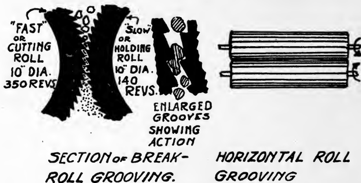
Fig. 10.—Section of Roller Mill.
