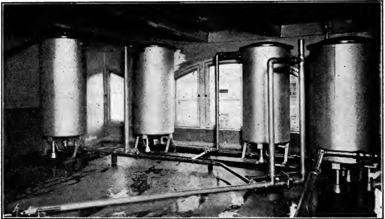
Fig. 53.—Holding Tanks. Milk heated to 145^{\circ} F. is conducted successively to four holding tanks where it is held for fifteen minutes in each tank. At a temperature of about 142^{\circ} F. it passes back through the pasteurizers and is rapidly cooled. (Courtesy of the Sheffield-Farms-Slawson-Decker Co.)
