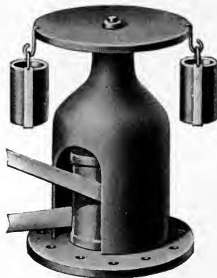
Fig. 44.—Early Experiment in Cream Separator. (Courtesy of the De Laval Cream Separator Co.)
