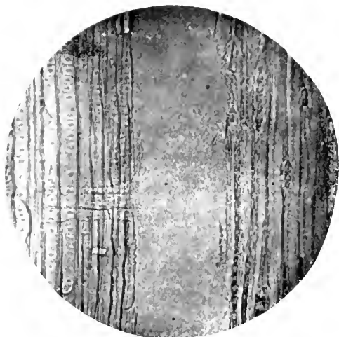
FIG. 208.—Pine Wood, \times 110 . Radial and tangential sections.
