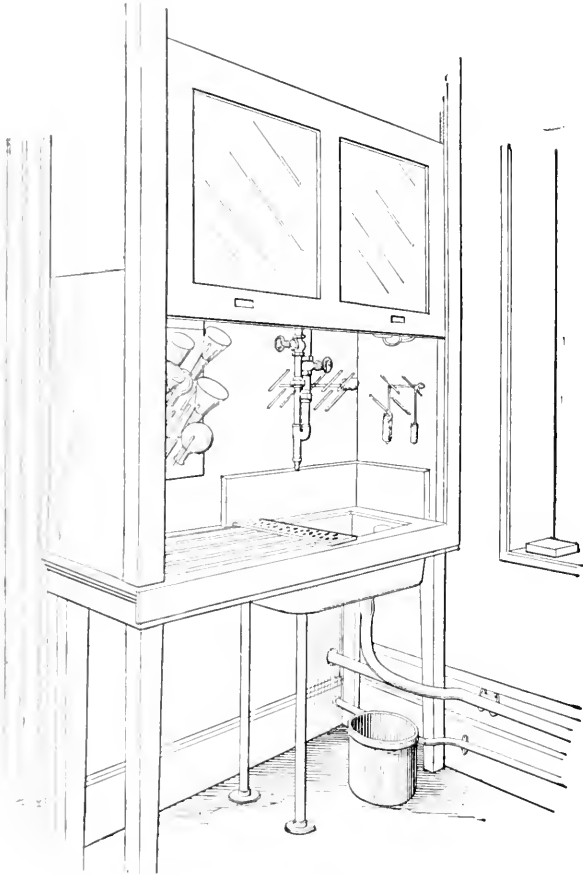
FIG. 4.—A Hooded Sink. An injector-like arrangement of steam and cold-water pipes furnishes water of any desired temperature.
