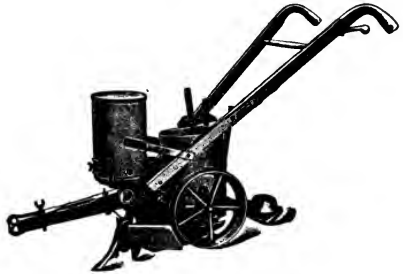
Improved cotton drill with fertilizer attachment
