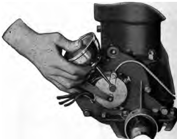
Figure 41.—Oiling the Commutator.
