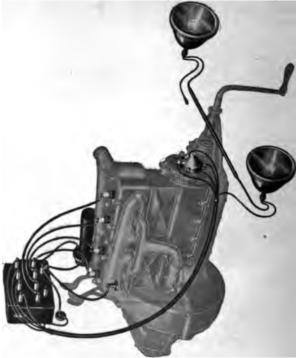
Figure 57.—Ignition and Lighting Parts on the Car.
