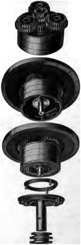
Figure 52.—Transmission and Clutch Partly Assembled
