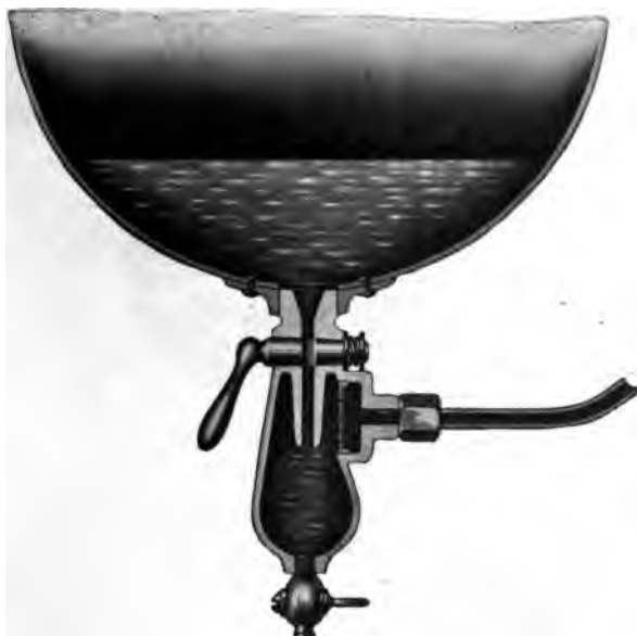
Figure 10.—Fuel Tank and Sediment Trap.
