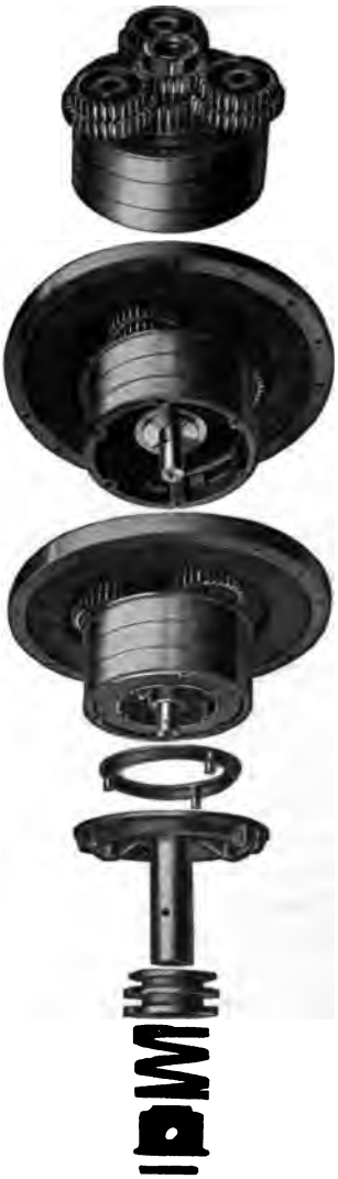
Figure 52.—Transmission and Clutch Partly Assembled
