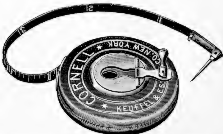
FIG. 5.—Tape for Measuring Girths and Diameters.
