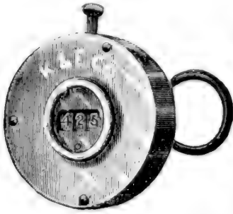
FIG. 37.—Tally Register. The box is carried within the palm of the hand and held by a ring through which the middle finger is passed. It counts from 1 to 999 and costs $2.50. (See Fig. 37.)
