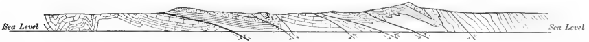
Fig. 243. — Geologic structure of the Appalachian region where extreme faulting has occurred. Length of section, 8½ miles. (Keith, U. S. Geol. Surv.)
