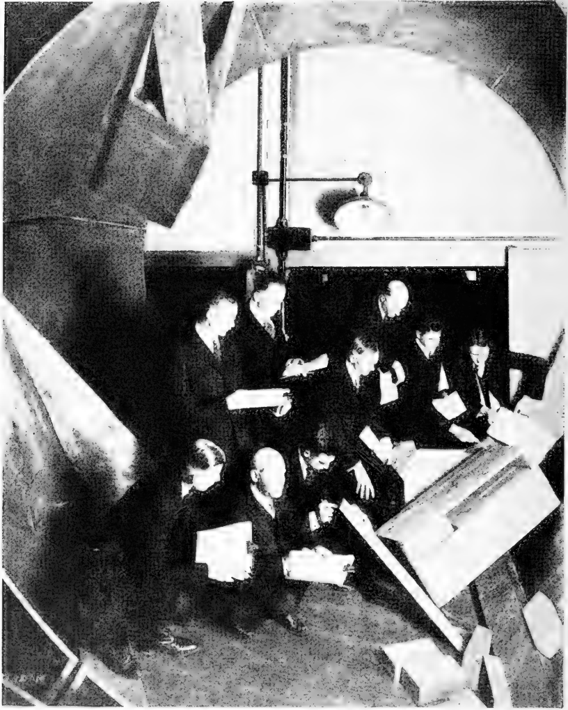
Classes in boxing and crating at the Laboratory make use of the 14-foot drum testing machine to investigate the serviceability of shipping boxes. The manufacturers and shippers in the group traveled an average of 5,000 miles each to attend the one-week course
