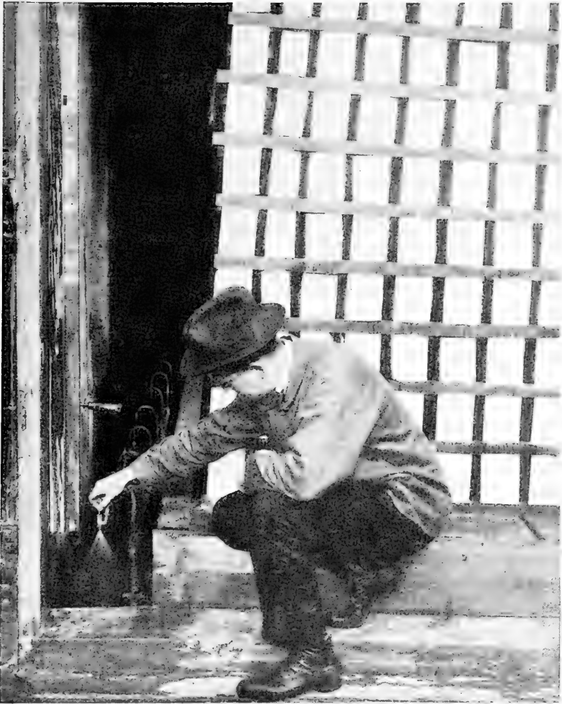
The distinctive feature of the Forest Service water-spray kiln is the control of the humidity in the kiln and, consequently, the drying rate of the lumber, by conditioning the air with sprays of water whose temperature is carefully regulated. The experimental kiln shown is drying oak bolster stock, which appears white because of the end dip used to reduce checking.
