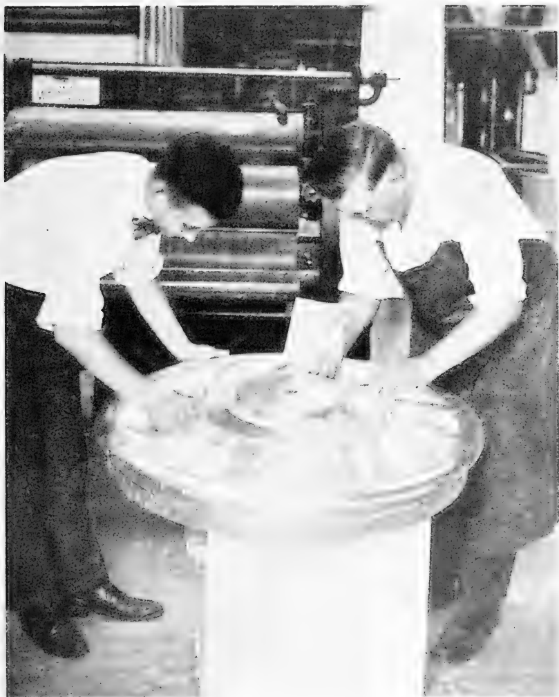
Wooden patterns for castings can be made practically moisture proof by an aluminum leaf coating and so prevented from warping, swelling, or shrinking. Car-wheel patterns protected in this way are now in use by several large foundries.
