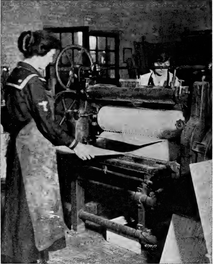
In the manufacture of water-resistant plywood with casein glue, the glue is applied cold to the veneer sheets by means of a mechanical glue spreader. The sheets are then placed one on top of another in a press.
