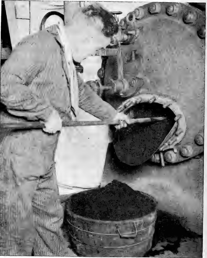
The first step in the manufacture of cattle food from sawdust is to cook the sawdust with dilute acid in a steam pressure cylinder. This converts a part of the wood into sugars and renders the remainder more digestible. Hydrolized sawdust is being successfully fed to cattle as a considerable part of their concentrate ration.
