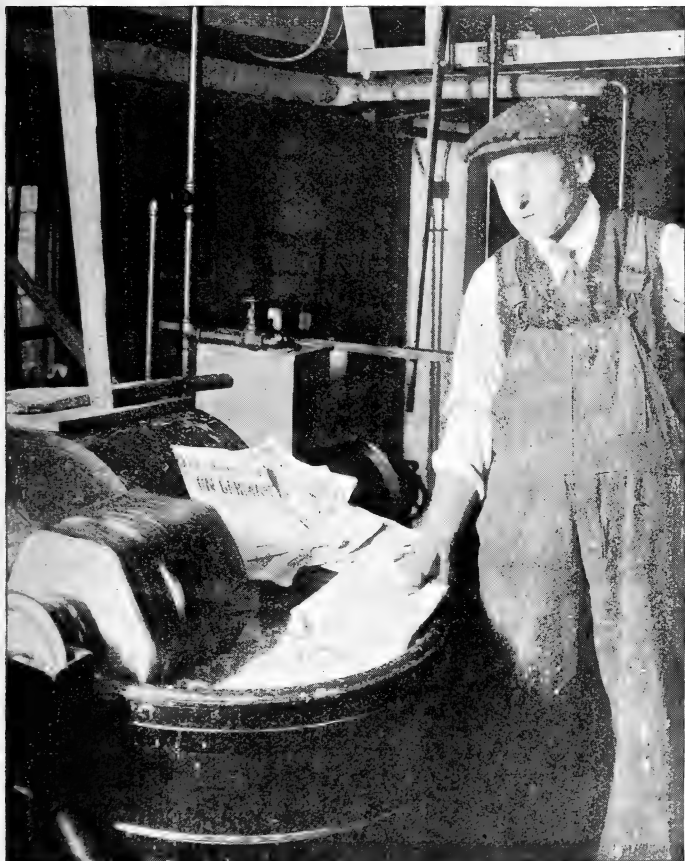
Old newspapers can be de-inked by the use of bentonite, a highly colloidal clay, to which the ink particles adhere after being loosened from the paper in the pulp beater. The pulp is then ready to be used again in the manufacture of newspaper.
