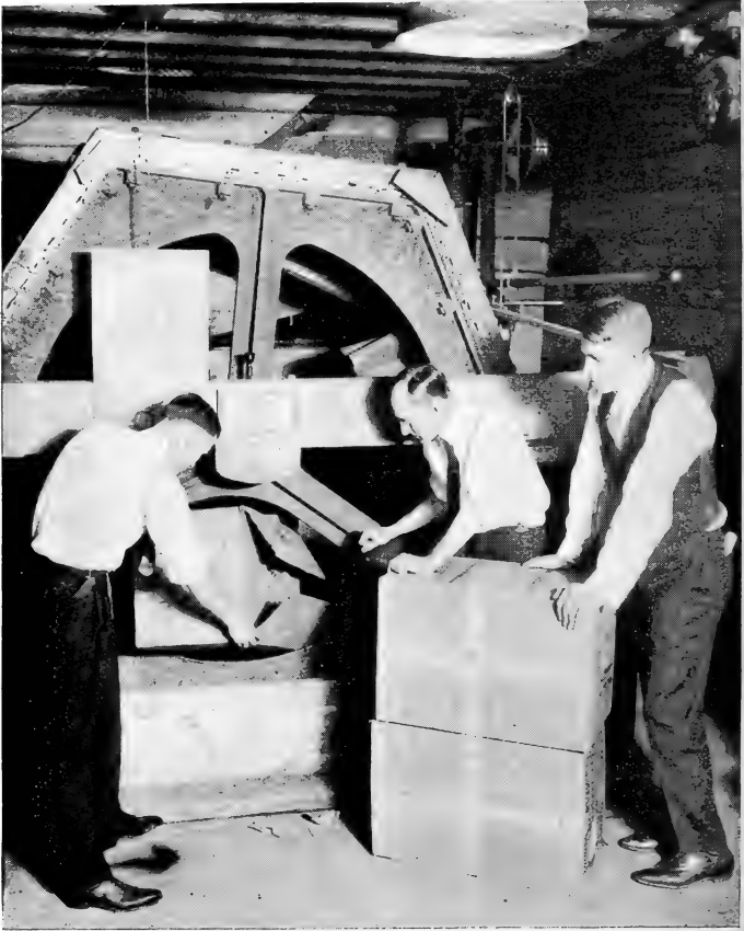
The drum-testing machine, developed by the Laboratory to stimulate the hazards of transportation, has become standard for shippers, packers, and manufacturers. The boxes shown are packed with electric-light bulbs. Four thousand dollars' worth of bulbs were furnished by the electric companies concerned for this series of tests to develop a better container.
