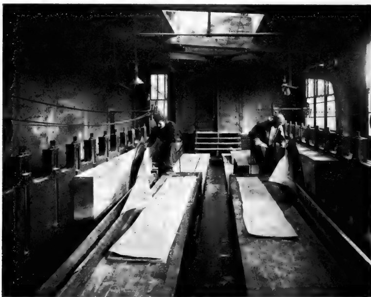
FIG. 20.—Making sawed veneers. Many of the finest veneers are made by this method.
