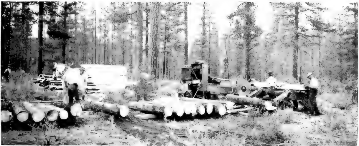
FIGURE 30.—Portable tie mill which cuts approximately 300 ties a day. Three men operate it—a sawyer, offbearer, and stacker. Four horses, used singly, yard logs from the woods.
