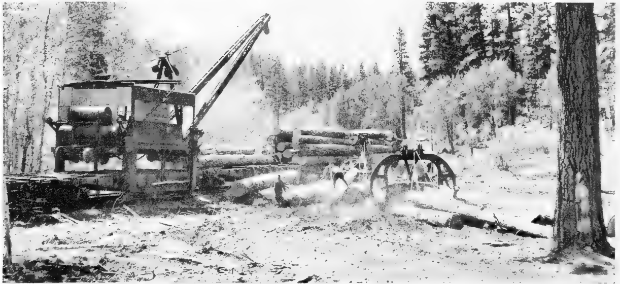
FIGURE 28.—Loading ponderosa pine logs on flat cars with gas “jammer.” Tractors with arches are used to bring logs to the landing.
