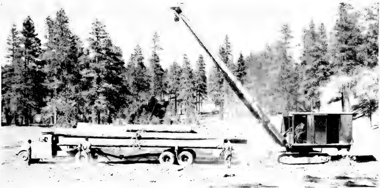
FIGURE 29.—Loading ponderosa pine logs on truck with a Diesel converted shovel loader.
