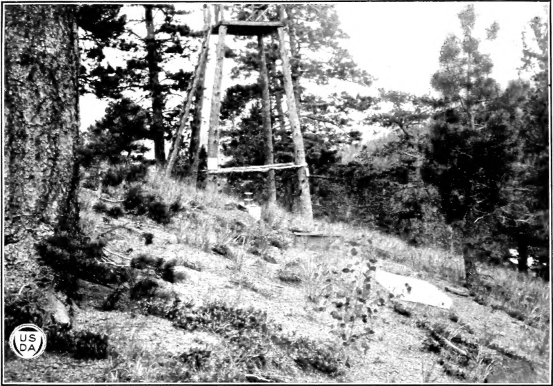
FIG. 1.—STATION F-2, SHOWING THE FOREGROUND SOIL WELL, THERMOMETER PIPES, AND EVAPORIMETER, AND IN THE BACKGROUND, TOWER ON WHICH OBSERVATIONS WERE MADE FROM 1910 TO 1912. JULY 7, 1918.
