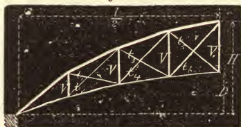
Upper Boom Loaded.
