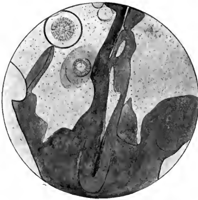
FIG. 1. Section from "yolk" in ordinary light. Dark portion opal; light portion, including spherules, chalcedony.
