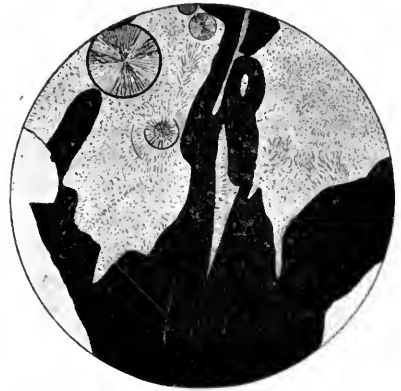
FIG. 2. Same in polarized light. The opal becomes black; the chalcedony shows a fibrous structure and the spherules interference crosses.
