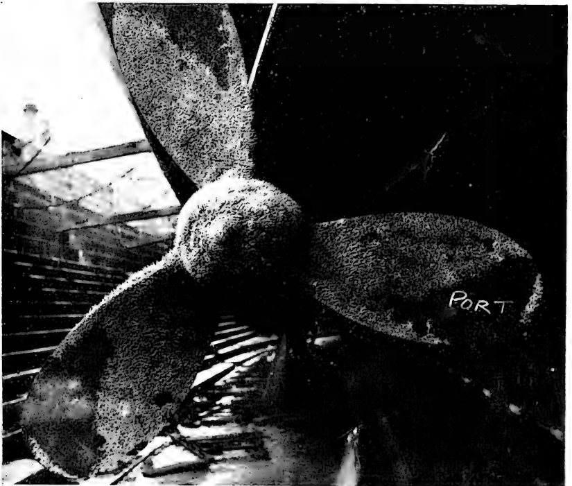
Fig. 18.—Fouling of propeller of H.M.S. Fowey by calcareous tubeworms. (Reproduced, by courtesy, from G. D. Bengough and V. G. Shephard, "The Corrosion and Fouling of Ships," Transactions of the Institution of Naval Architects , 1943, vol. 85, p. 1.)
