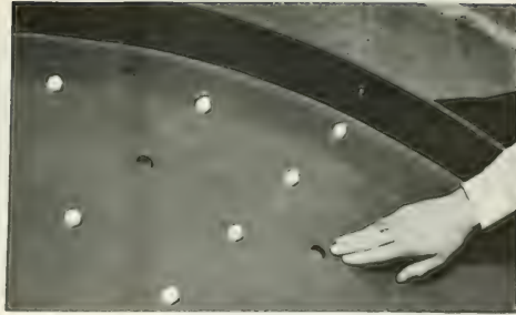
b. Footing Underside Showing Keying Edge
