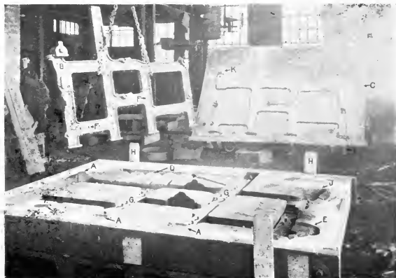
FIG. 21.—DRAG OF WIRE CLOTH LOOM FRAME ON FLOOR. COPE IS STANDING AGAINST WALL.
