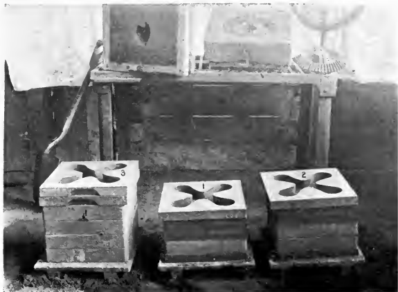
FIG. 5.—MOLDS WEIGHTED FOR POURING.
