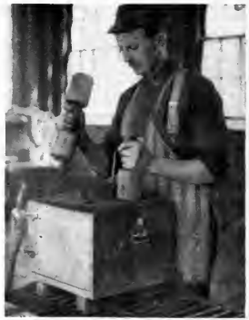
FIG. 4.—BUTT-RAMMING THE SURFACE OF THE MOLD.
