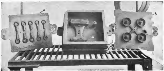
FIG. 127.—GATING PATTERNS ON MATCH-PLATES.
