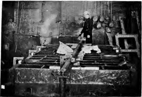
FIG. 22.—WIRE CLOTH LOOM FRAME MOLD CLAMPED READY FOR POURING AND BOUND DOWN WITH BINDER.
