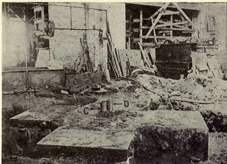
FIG. 80.—PROPELLER MOLD AFTER REMOVING WEIGHTS AND CLAMPS AND JUST BEFORE SHAKING-OUT. THE RISER AS SHOWN AT C AND D IS A PIPE PLACED OVER THE VENT IN THE CORE.
