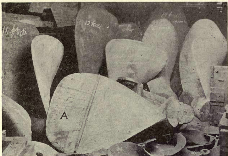
FIG. 82.—PATTERNS FOR A WIDE ASSORTMENT OF PROPELLERS THAT CAN BE MOLDED IN ONE SET OF FLASKS.
