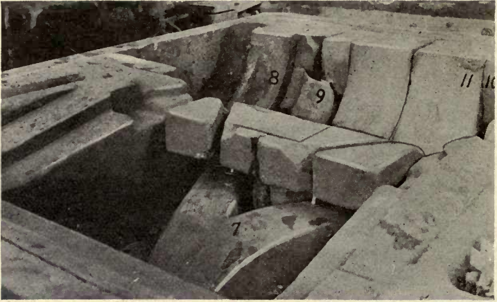
FIG. 119.—CHEEK PART OF THE MOLD, SHOWING Y-SHAPED EXHAUST CORE AT 7.
