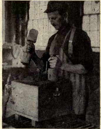
FIG. 4.—BUTT-RAMMING THE SURFACE OF THE MOLD.
