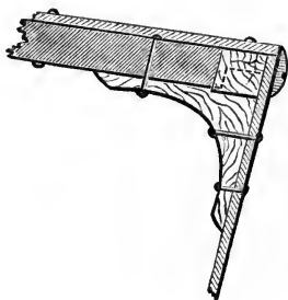
HOW TO SECURE ENDS OF FORE AND AFT DECK-RAFTERS, AS WELL AS OF GUNBEAM. (Side view.)
