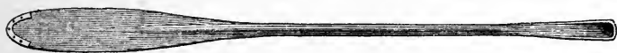
LONG ASH PADDLE, OF IMPROVED SHAPE, FOR GENERAL USE IN SHALLOW WATERS ABOARD FOWLING-PUNTS WHEN NOT SETTING TO FOWL.
