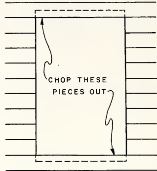
FIG. 12-7 SHEATHING AT TOP AND BOTTOM OF OPENING
