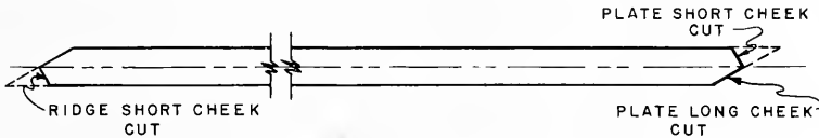
FIG. 18-11 SHORT CHEEK CUTS OF VALLEY RAFTER
