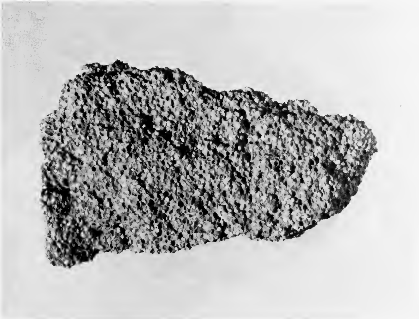
FIG. 69. Hand specimen of the oolitic rock. The oolites are loosely cemented and they can be freed easily. Natural size.
