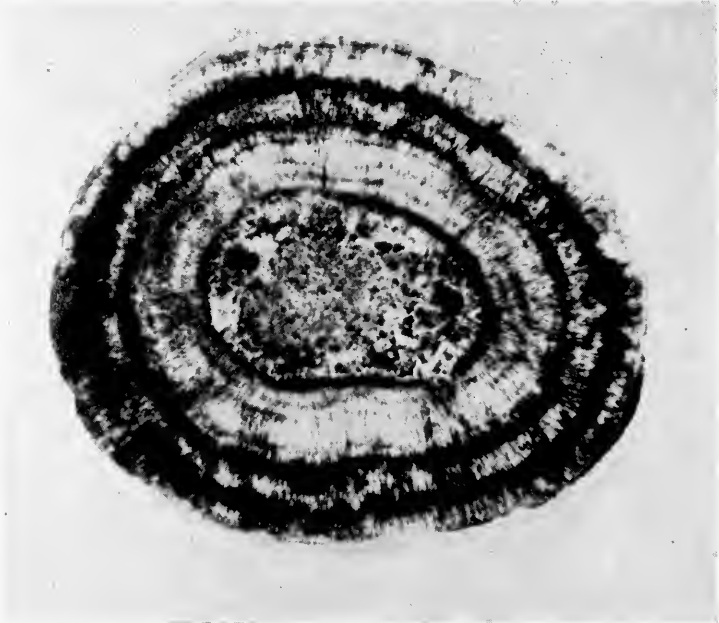
FIG. 71. Section of individual oolite, showing concentric and radial structure. Crossed nicols. \times 60 .
