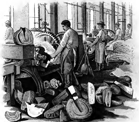
FIRST PROCESS.—GRINDING CRUDE RUBBER.
