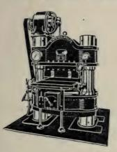
In the lead mold process the plastic medium used is a soft thin sheet of what is called "impression lead," .040 inches thick, instead of wax, and the lead is placed on top of the original to be duplicated, instead of vice versa, as in the wax-molding process. No "building-up" nor "black-leading" is necessary.
