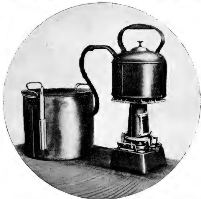
Apparatus for bottling fruits. The bottles of fruit are placed in the steriliser (on left) and steam is introduced from the kettle through the tube
