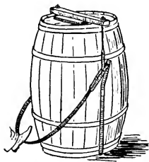
FIG. 16—ORDINARY LEVER PRESS FOR APPLE BARREL
