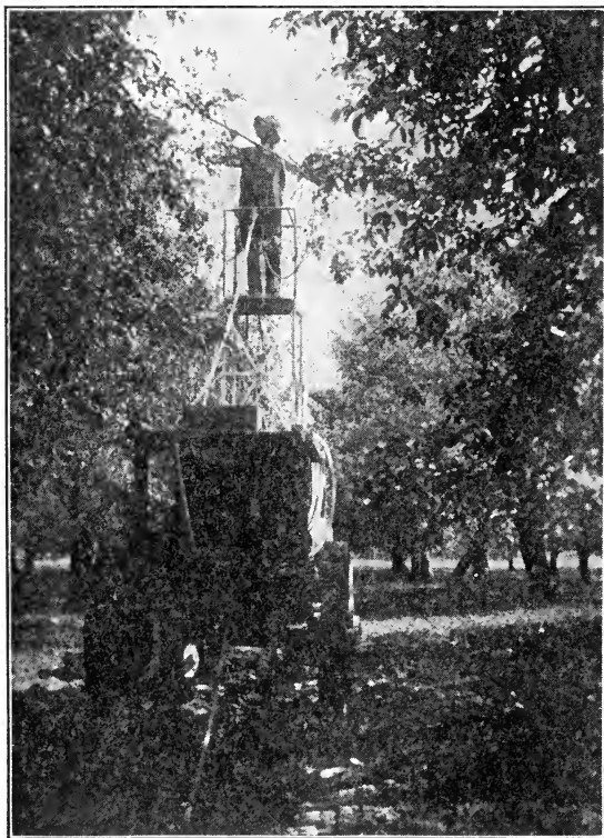
A POWER SPRAYER ADAPTED TO LARGE TREES. A gasoline engine gives uniformly high pressure.
