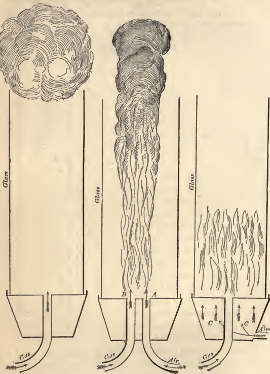
Figs. 22, 23, 24.—Supply of air to burn gas.
