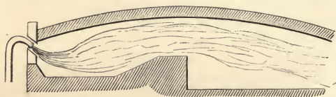
Fig. 140.—Crampton's Powdered Fuel Furnace.
