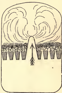
Fig. 29.—Air through orifices in the fireplace.
