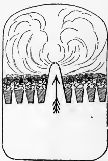
Fig. 29.—Air through orifices in the fireplace.
